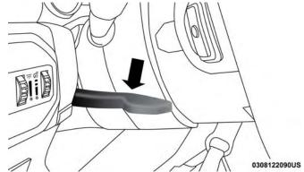
Tilt/Telescoping Steering Column Lever
