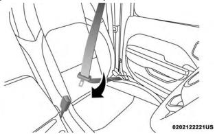
**Inserting Latch Plate Into Buckle**
