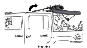
**NOTE:** If leaving the soft top in the Sunrider position, secure the top by using the two hook-and-loop fasteners provided in the center console.
