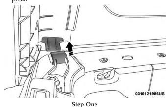
2. Undo the hook-and-loop fastener located at the upper front corner of each quarter window.
