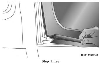
4. Remove plastic retainer from the bottom to the top of the front window.
