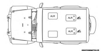
ALR — Switchable Automatic Locking Retractor (Two-Door Models)
