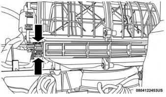
Air Filter Retaining Tabs
