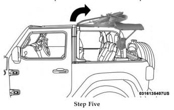
**NOTE:** If leaving the soft top in the Sunrider position, secure the top by using the two hook-and-loop fasteners provided in the center console.
