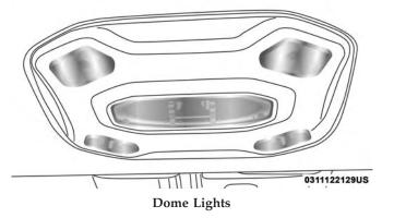
When a door is open and the interior lights are on, rotating the dimmer control to the extreme bottom position will cause all the interior lights to turn off. This is also known as "Party" mode because it allows the doors to stay open for extended periods of time without discharging the 3 vehicle's battery.
