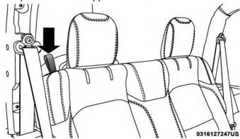
Rear Head Restraint Folding Strap Location
