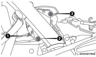
Lift Assist Mechanism In Place
