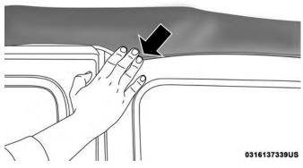
Firmly Secure Hook-And-Loop Fastener
