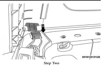
3. Engage the plastic retainers on the front of the window, followed by the retainers along the bottom. Repeat on the other side.
