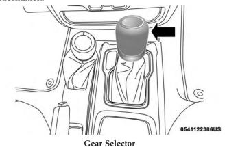
**NOTE:** If the gear selector cannot be moved to the PARK, REVERSE, or NEUTRAL position (when pushed forward), it is probably in the AutoStick (+/-) position (beside the
