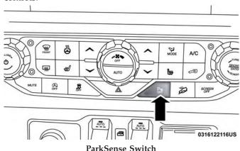
When the ParkSense switch is pushed to disable the system, the instrument cluster display will show the "PARKSENSE OFF" message for approximately five seconds. Refer to "Instrument Cluster Display" in "Getting To Know Your Instrument Panel" for further information. When the gear selector is moved to REVERSE and the
