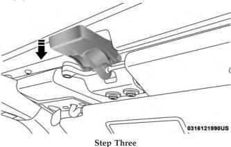
4. From both the left and right sides, lift up on the #1 Bow of the soft top to start the operation.
