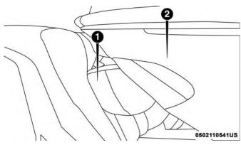
Car Seat With Head Restraint Folded
