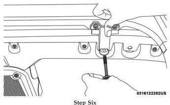
Door Frame Installation Two Door Models — If Equipped
