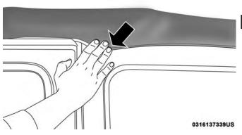
Firmly Secure Hook-And-Loop Fastener
