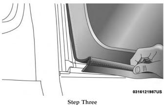
4. Remove plastic retainer from bottom to top of the window.
