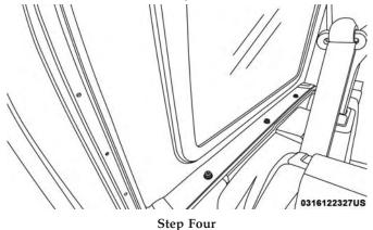
5. Open the swing gate all the way to ensure clearance of the rear window glass. Lift the rear window glass.
