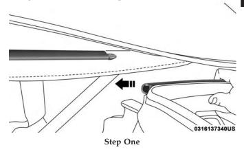
2. Place the top of the quarter window pillar into the top cover, and insert the bottom tab into the clip.
