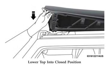
6. From inside the vehicle, pull the handle on the header latch downward to engage the hook into its receiver. Repeat on the other side.
