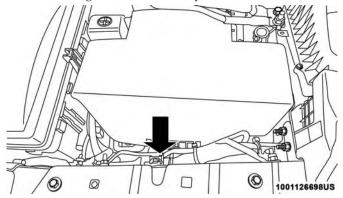
Auxiliary Switch Connections - Under Hood
