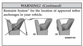
1. Look behind the seating position where you plan to install the child restraint to find the tether anchorage. You may need to move the seat forward to provide better access to the tether anchorage. If there is no top tether anchorage for that seating position, move the child restraint to another position in the vehicle if one is available.
