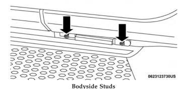
2. Remove both nuts from the underside of the vehicle for each bracket.
